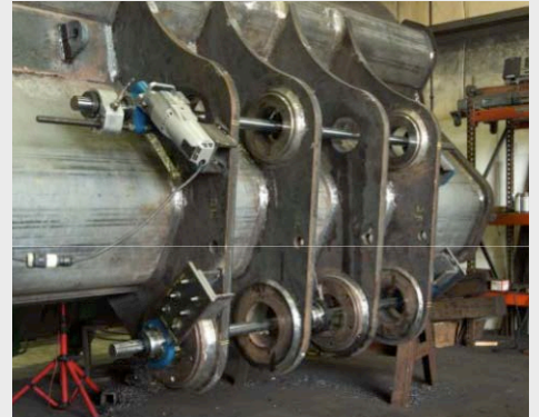
*Pictures of actual portable line boring machine in use
